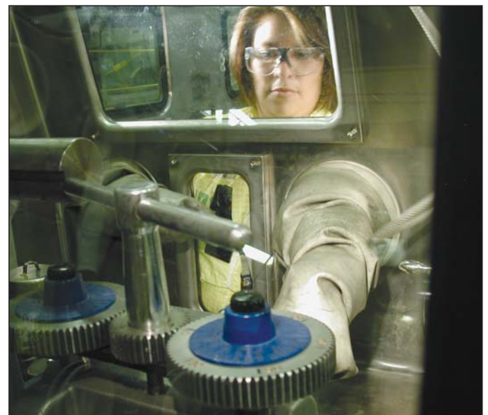
Above: Claudette Trujillo, a materials accountability specialist in Nuclear Materials Science (NMT-16), assists with rolling the spiked plutonium on a laboratory-scale rolling mill (foreground). Photo by Joe Martz, NMT-16
