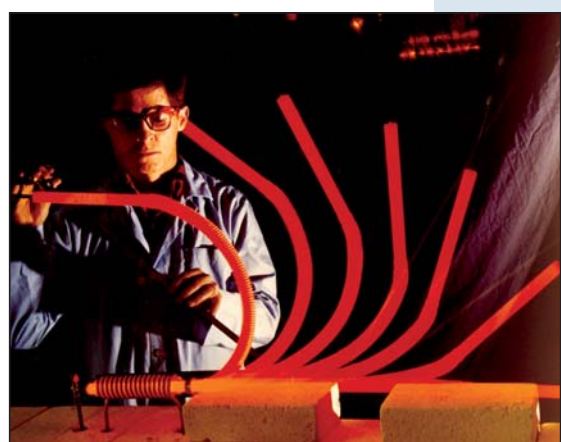
Prototype testing of a flexible heat-pipe design.
