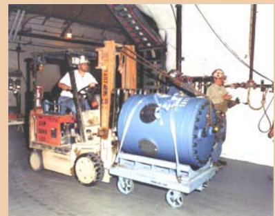
Confinement vessel used in explosive tests at Nevada Test Site aimed at guarding the nuclear stockpile
