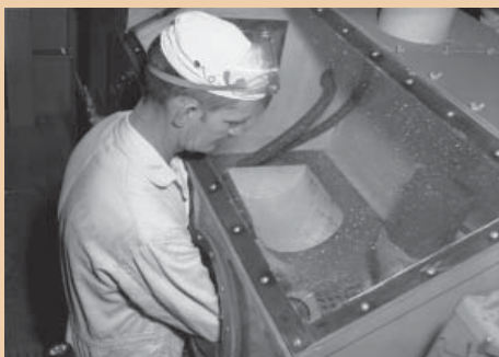
A chemical worker at Fernald uses a glovebox to sample uranium material, April 1970
