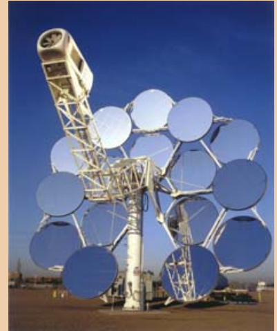
Solar technology uses mirrors to focus sunlight onto a thermal receiver
