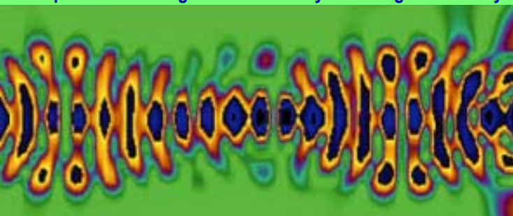
Electric field in a 2D photonic crystal waveguide
