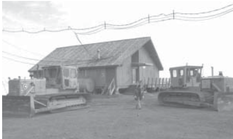
A McMurdo Station worker inspects two older D-8 Caterpillar bulldozers in front of the Chalet administration building. The D-8s have not been built since 1963 and have been working in Antarctica for 50 years.
