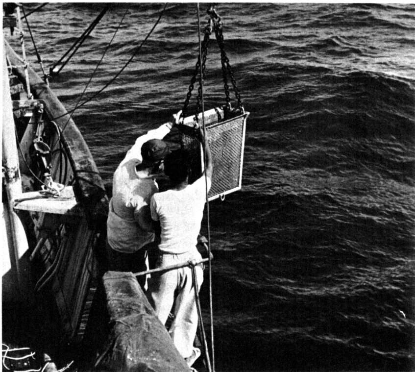
Figure 19.— Scientist from India and U.S. colleague, lowering a dredge from the Anton Bruun, U.S. biological research ship during the International Indian Ocean Expedition.
