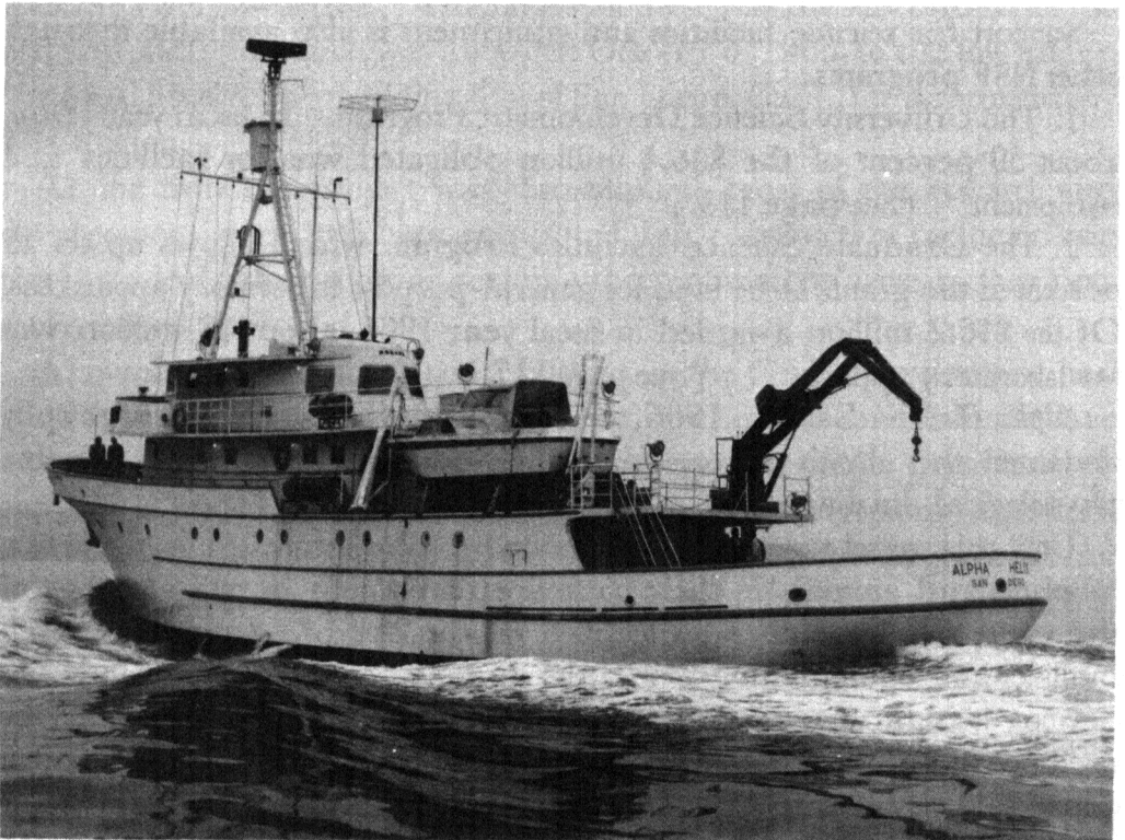
Figure 16.—Designed for marine physiological investigations, the 133-foot floating laboratory, Alpha Helix , was constructed under an NSF Specialized Science Facility grant. The vessel provides seaborne scientists with complete facilities and equipment for studying plants and animals in their natural environment.
