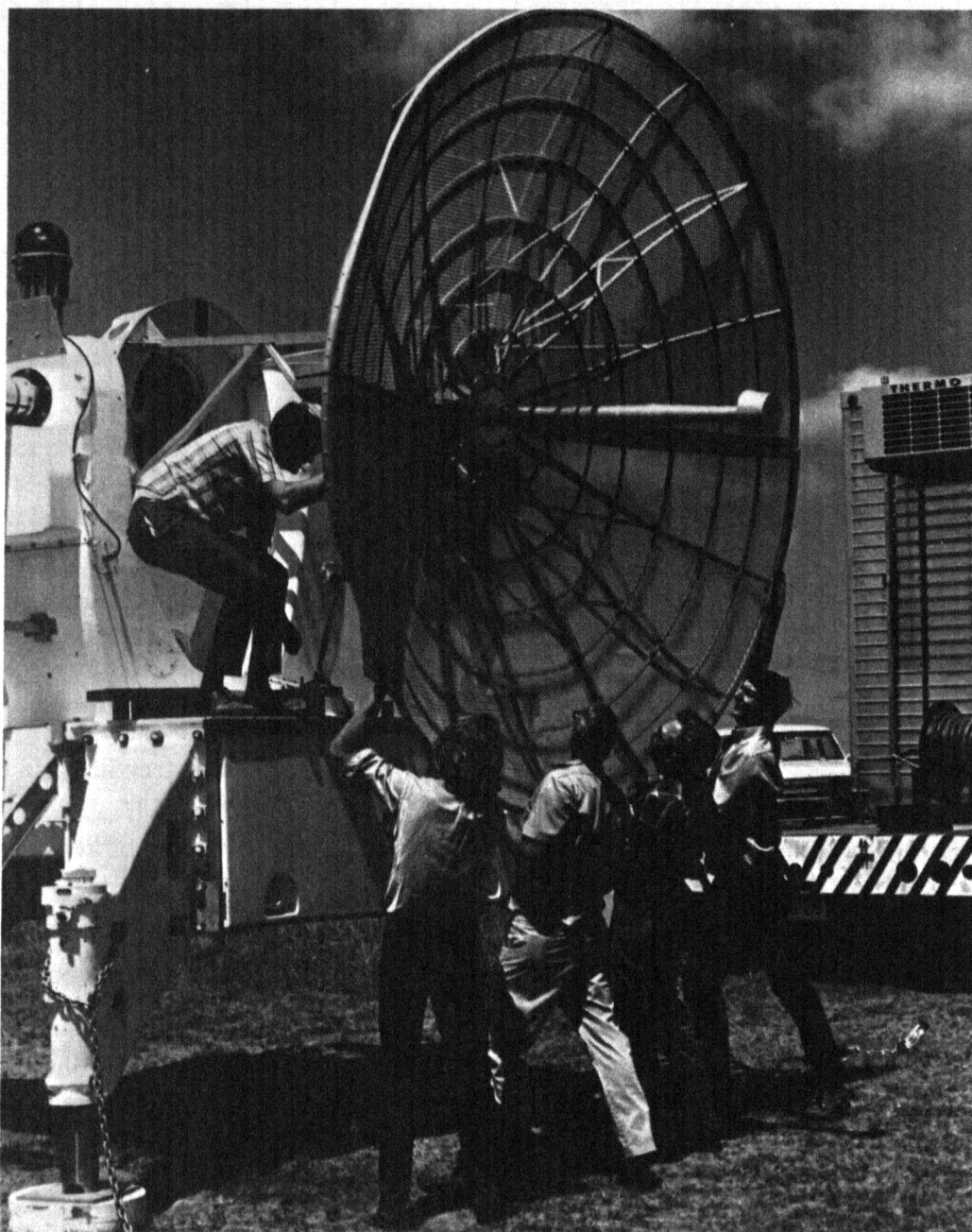
NCAR technicians set up coherent cloud physics radar near Grover, Colo., for use in the National Hail Research Experiment. Radar is used to probe the growth, structure, and motions of thunderstorms. (Photo NCAR)
