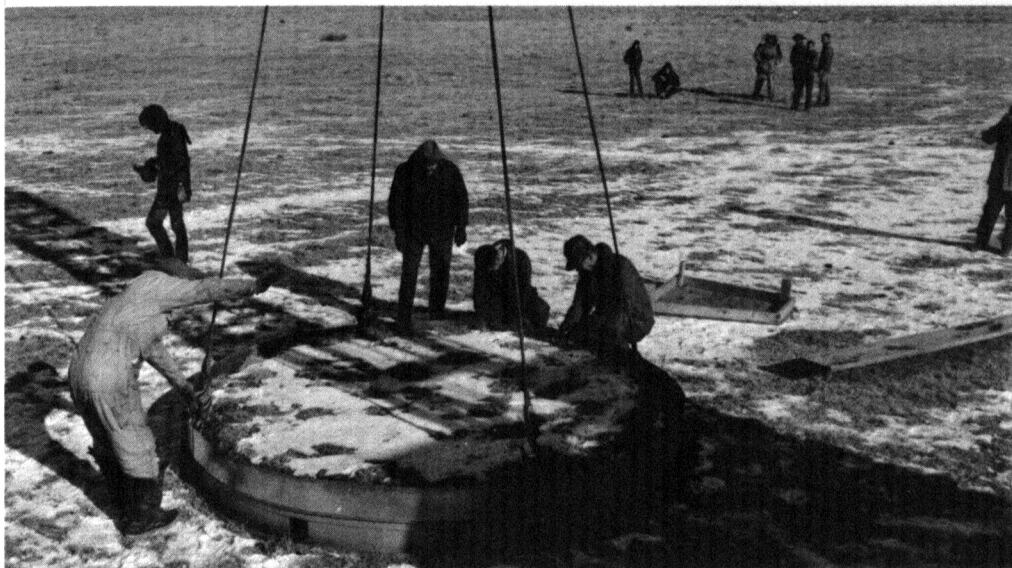
Lysimeter is large core of several tons of prairie soil and sod which can be weighed accurately to measure uptake and loss of water. In place, the core is not separated from surrounding plant life. (Photo Colorado State University)
