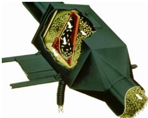
Figure 2. Diverter-Type sampler installed in spout.
