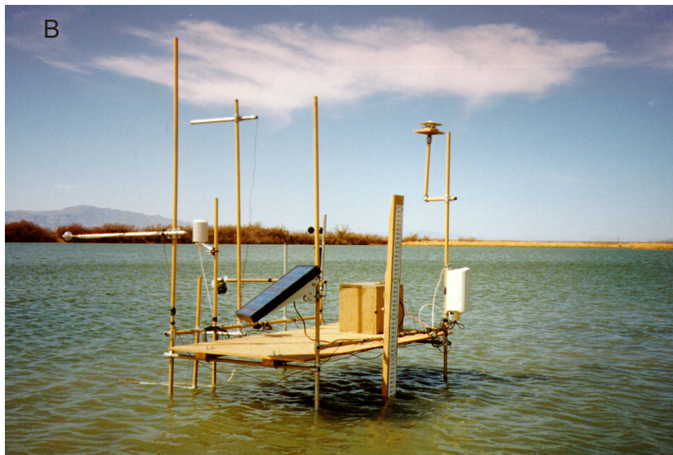
Figure 9. Typical instrument installations used to determine evapotranspiration (ET) from Ash Meadows area, Nevada. (A) LCFLAT site (pl. 1, table 6) established over moist bare soil (MBS, table 3). Vegetation is sparse and consists primarily of the bunchgrass, alkali sacaton ( Sporobolus airoides ). Soil is encrusted with thin layer of salt deposits. (B) PRESVR site established over open water (OWB, table 3).
