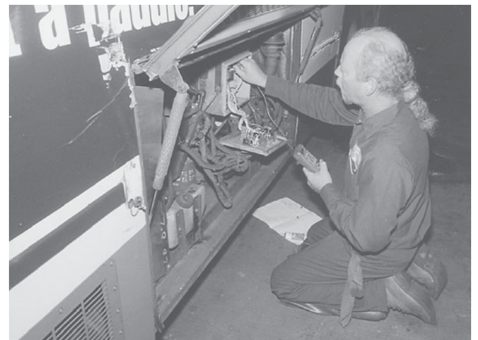
Diesel service technicians use a variety of testing equipment to pinpoint and analyze malfunctions in electrical systems and engines.
