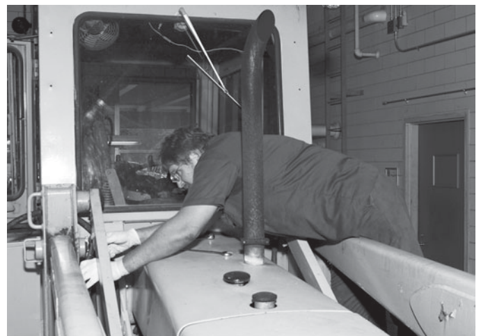
With many types of modern heavy and mobile equipment, technicians can plug hand-held diagnostic computers into onboard computers to diagnose components needing adjustment or repair.
