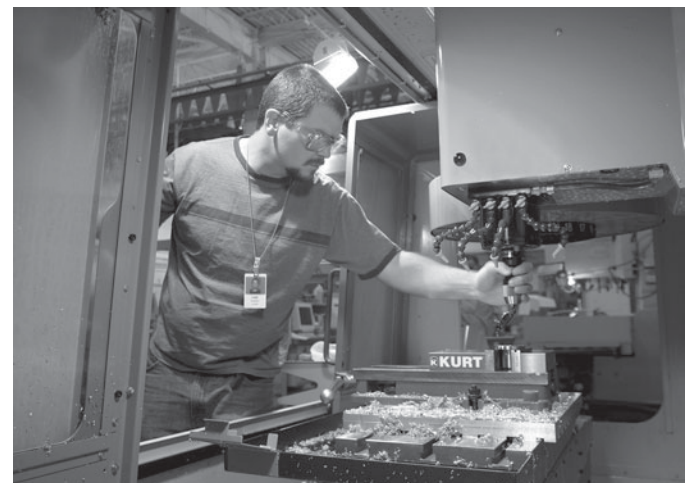
Machinists replace worn cutting tools.
