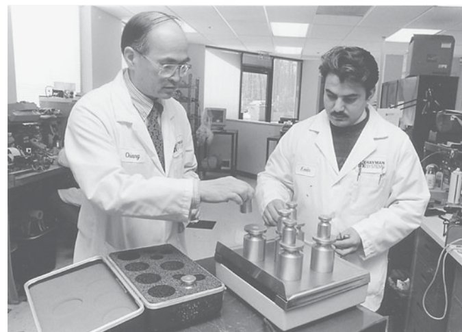
Inspectors calibrate scales.
