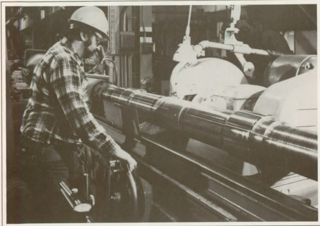
Illustration 10. Juniata Shops, Axle Finishing Shop (in Machine Shop No. 1), Journal Lathe. Photograph by Jack E. Boucher, 1988. Courtesy of Historic American Engineering Record, Washington D. C.
