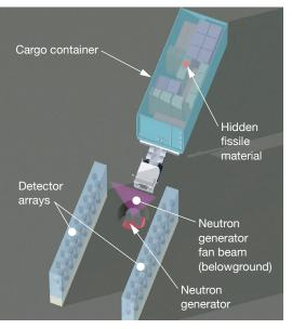
The design for the detector system calls for a belowground neutron generator that would bathe containerized cargo with neutrons. Interaction of the neutrons with fissile material inside the container would produce fission, followed by delayed gamma rays detected by an array of liquid scintillators as the container moves through the system.
