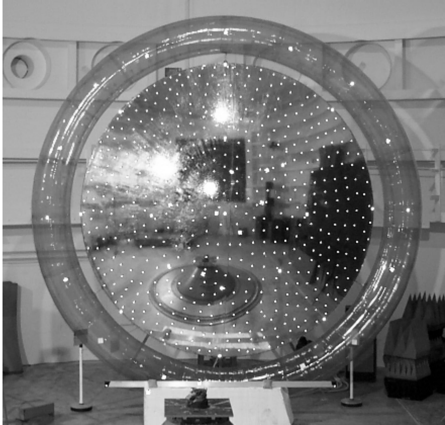
Figure 1: The 5m concentrator mounted in the 16m vacuum chamber. The rear, convex surface of the concentrator is shown, and this is the surface measured in this research.
