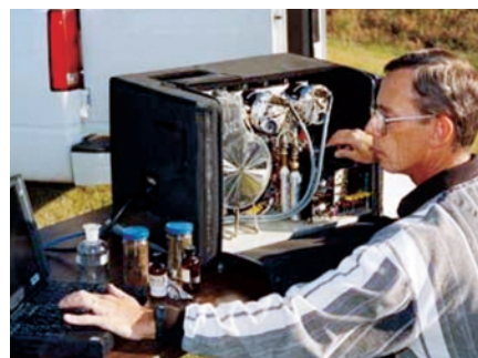
Forensic Science Center chemist Del Eckels uses the 28-kilogram portable gas chromatograph–mass spectrometer that fits inside a wheeled suitcase. The portable unit, comparable in sensitivity and selectivity to much larger and heavier units, permits fast on-the-scene chemical analysis.
