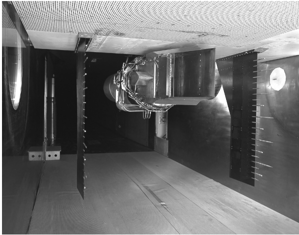
Figure 11. Inlet unstart experiment hardware installation with instrumentation struts.
