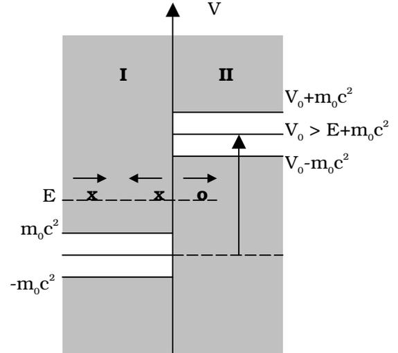
**Figure 3.** Energy Continuum of the Dirac Equation at a Potential Barrier.<sup>34</sup> (x) = particle, (o) = antiparticle
