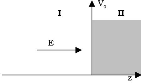
**Figure 2.** Particle incident on a potential step.
