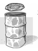
Cut open the drum. Remove and save the top cutaway piece.
