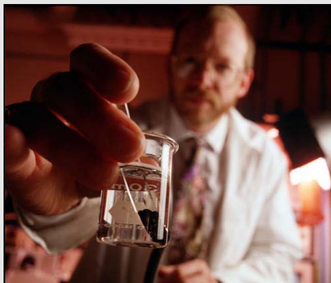
Photoelectrochemical water splitting: Using a photovoltaic cell/electrolyzer submerged in an alkaline aqueous solution to produce hydrogen. (Photographer: Richard Peterson)
