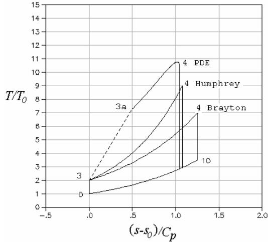
Figure 1. Ideal Cycle Analysis for the Brayton, Humphrey, and PDE Processes.<sup>2</sup>
