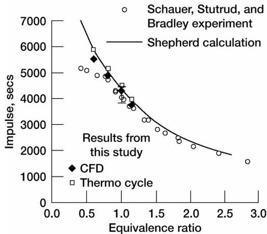
Figure 6. Comparison of analyses with WL data, hydrogen-air.<sup>7</sup>
