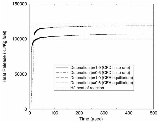
Figure 5. Sensible heat release for hydrogen-air, equilibrium, and finite rate reaction (lower curve is stoichiometric).<sup>6</sup>
