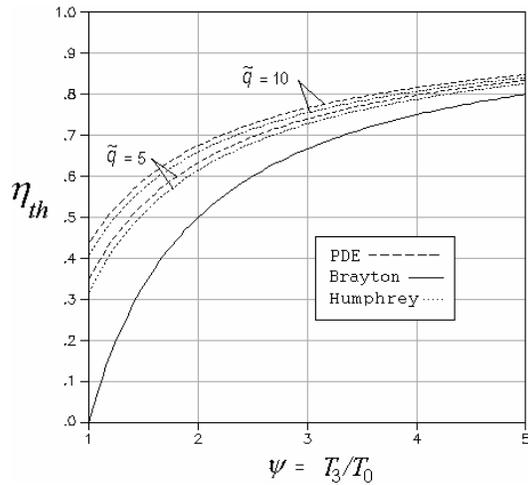
Figure 2. Thermal efficiency of the Brayton and PDE Cycles for equal values of  $\tilde{q}$ .<sup>2</sup>
