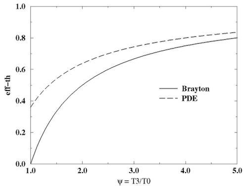
Figure 3a. Thermal efficiency for unequal values of  $\tilde{q}$ , stoichiometric propane-air.<sup>3</sup>
