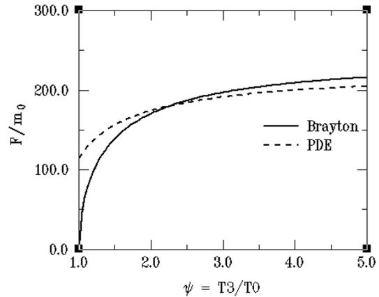
Figure 3b. Specific thrust for the PDE and Brayton Cycles versus temperature ratio, stoichiometric propane-air.<sup>3</sup> (units same as in figure 4)
