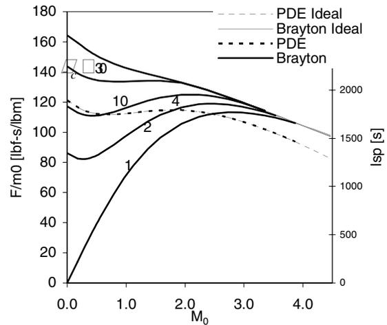
Figure 4. Specific thrust versus Mach number for Brayton and PDE cycles, stoichiometric propane-air.<sup>5</sup>
