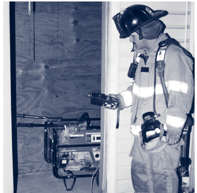
FIGURE 1. A firefighter uses a portable meter to measure the carbon monoxide (CO) level after CO exposure caused by a generator forced evacuation of an apartment building — Charlotte, North Carolina, 2003
