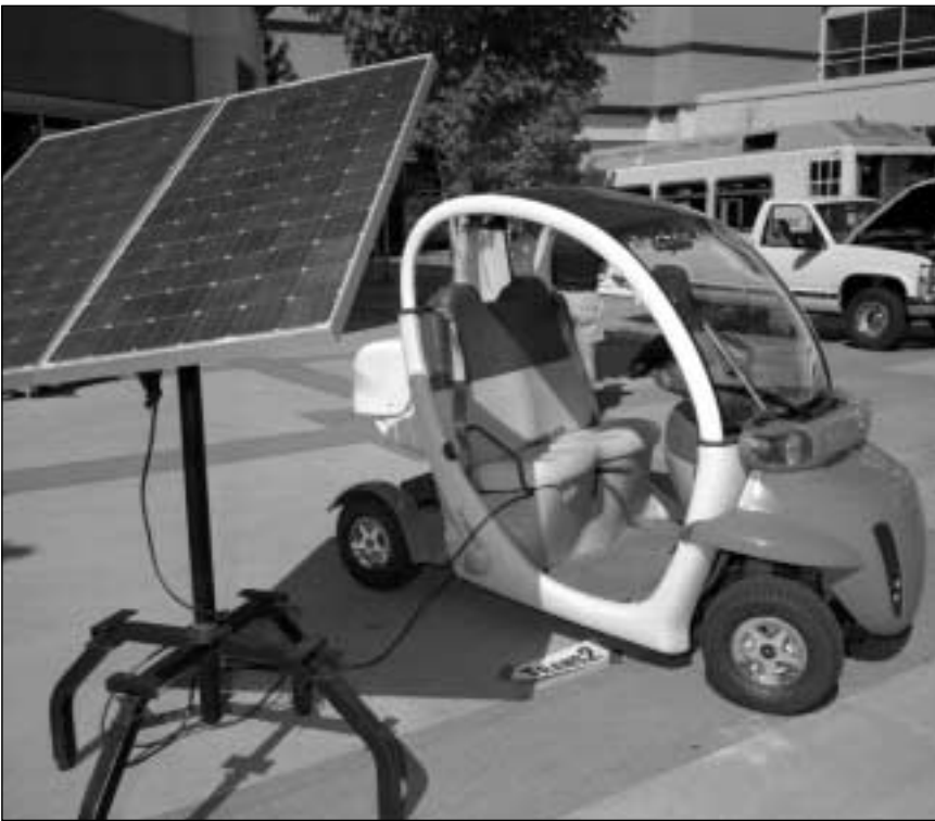
The sun's energy, via a photovoltaic module, is used to recharge this electric vehicle.
