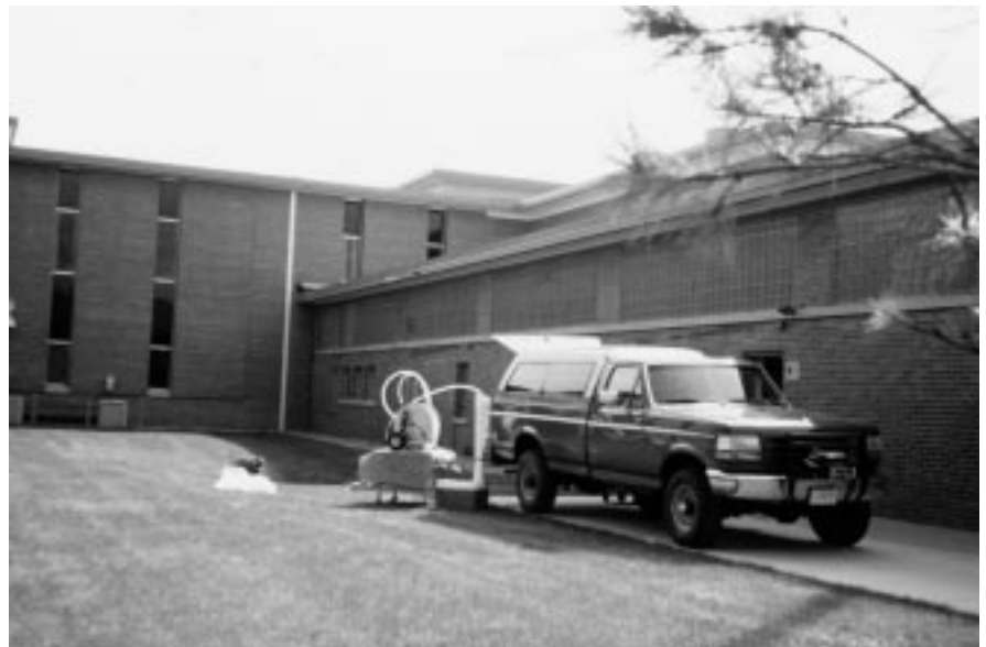
An "equipment blank" sample is prepared at the USGS preparatory lab in Denver after ground-water sampling at Deer Trail by using the large submersible pump and all the equipment routinely used at the field site. This blank does not represent wind-born contamination at the field site.
