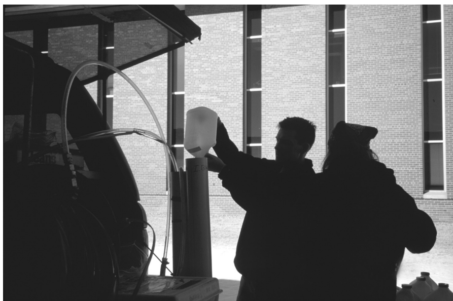
The ground-water “equipment blank” sample also is processed in the back of the sampling truck, but the truck is parked in Denver at the USGS preparatory laboratory. The “equipment blank” sample is designed to indicate contamination from the sampling equipment only, not the field site.
