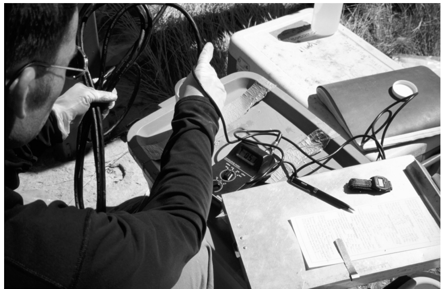
Quality assurance of the continuous-recorder sites includes calibration checks at the field site on all the sensors each year.
