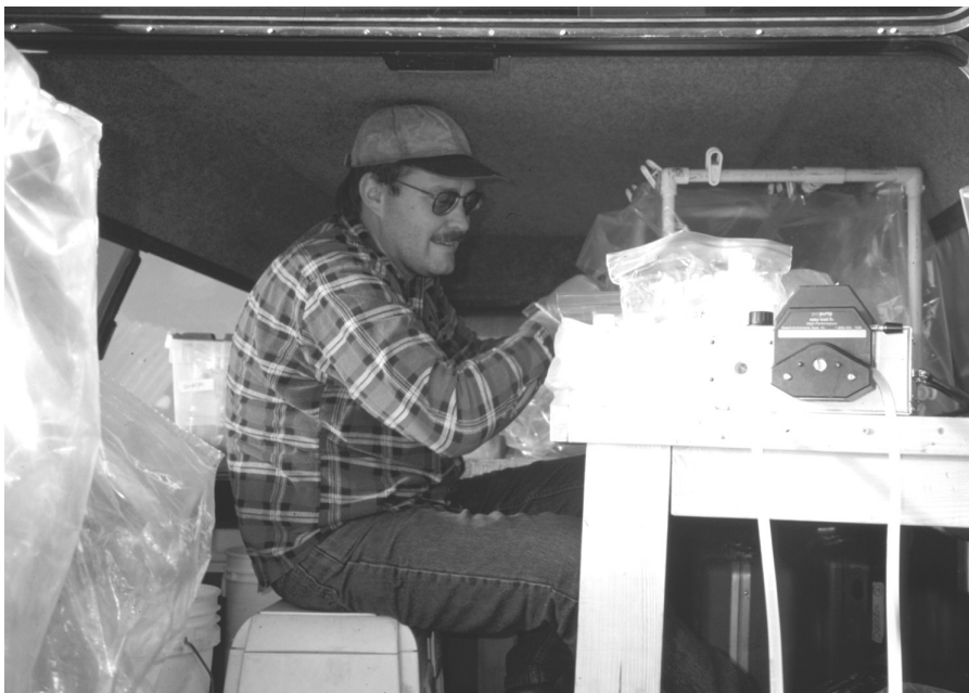
USGS ground-water samples are collected by pumping water into a special “clean room” chamber inside the back of the truck at the field site.
