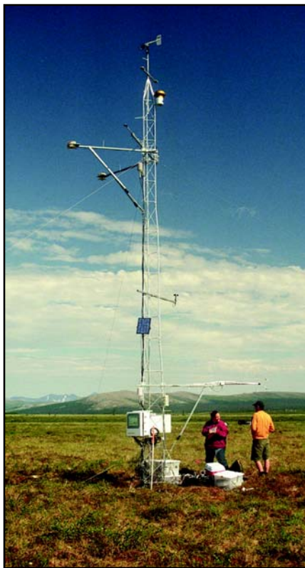
An eddy flux tower used to measure the weather and the flux of CO 2 and moisture from the tundra to the atmosphere.
