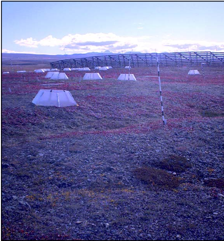
A set of ITEX cones on the tundra near Toolik Lake, Alaska. In the background is a snow fence designed to test the effect of increased snow on the tundra.
