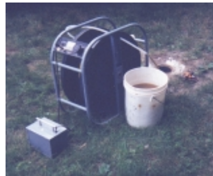
Sampling ground water at a monitoring well with an electric submersible pump (photograph by Stephen Garabedian, U.S. Geological Survey).
