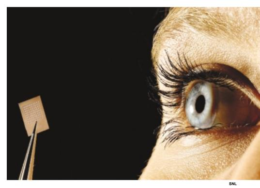
**Artificial retina:** This project, funded by a \$9 million, three-year grant from the Office of Science, will build a prototype that creates 1000 points of light through 1000 tiny microelectromechanical systems (MEMS) electrodes. The tiny electrodes may eventually be positioned on the retinas of those blinded by diseases such as age-related macular degeneration and retinitis pigmentosa to help them see again.
