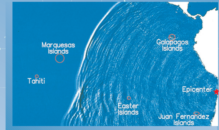
BELOW: Model of the tsunami in the south-east Pacific, nine hrs after its generation.
