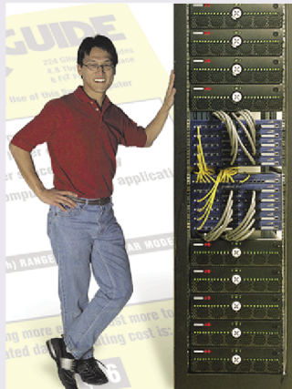
Green Destiny —The world's most efficient supercomputer, occupies less than 6 square feet and draws no more than 5.2 kilowatts of power
