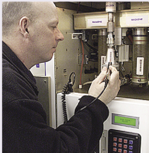
BASIS —Biological Aerosol Security and Information System to detect and identify airborne microorganisms
