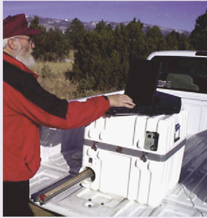
CARISS —Computational Analysis by Raman-Integrated Spark Spectroscopy, an integrated elemental and compositional analysis of material at close, standoff, and remote distances
