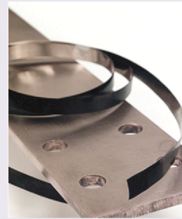
Flexible Superconducting Tape —Carries high currents in high magnetic fields at liquid-nitrogen temperatures
