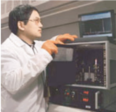
Yixiang Duan adjusts a filter in his portable air-particulate monitor.
