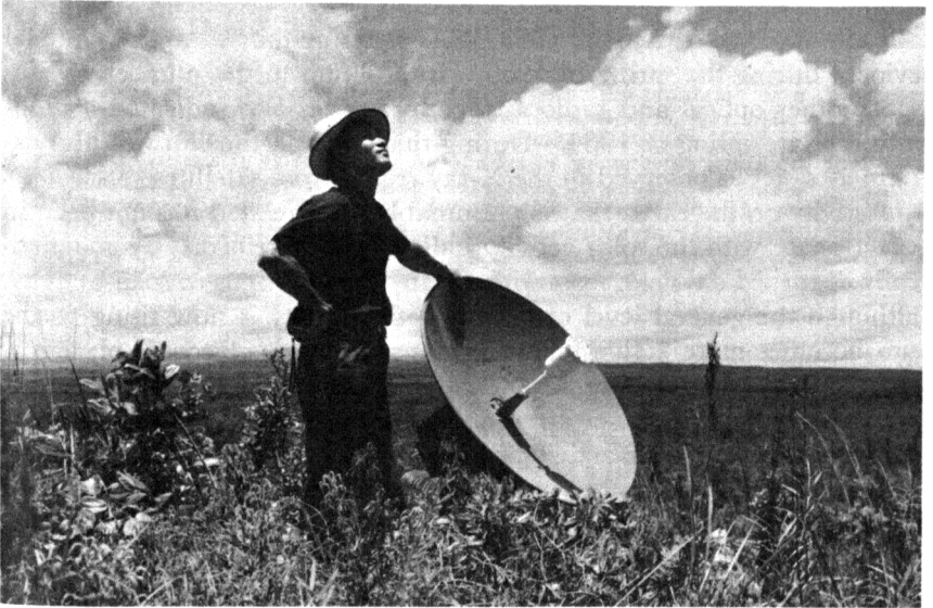
Figure 21. — Japanese radiosonde receiving antenna being used on Mount Mauna Loa, Hawaii, as part of a joint study by United States and Japanese scientists of warm rainfall mechanisms. This research was carried out as part of the United States-Japan Cooperative Science Program.
