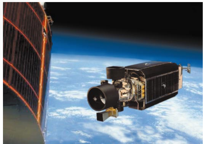
Figure 1. In this artist's rendering, a MicroSat gets a close look at a larger satellite. The goal is for the MicroSat to rendezvous with a satellite, inspect it, dock with it, service it, and verify its performance. It will look for signs of wear, including atomic oxygen and ultraviolet surface damage, micrometeoroid impacts, and debris cloud generation from leaks or other deterioration. These data can be stored on board or forwarded to ground control through an Ethernet connection.
