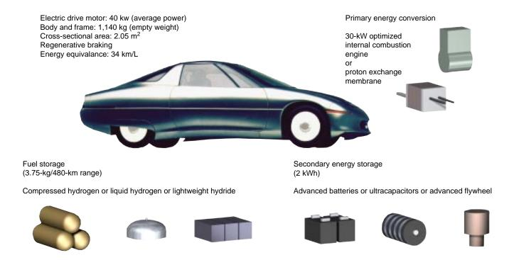
Figure 1. The Laboratory's hydrogen-fuel feasibility study based its analysis on a light-duty hybrid-electric vehicle with an internal combustion engine/generator or a proton-exchange fuel cell using hydrogen fuel in a variety of physical or chemical forms—e.g., compressed gas, cryogenic liquid, or hydrides. The vehicle has a 3.75-kg (8.3-lb) fuel storage capacity and a driving range of 480 km (300 miles) and gets gasoline energy-equivalent mileage of 34 km/L (80 mpg).
