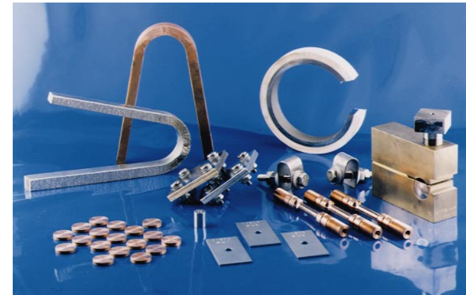
Figure 6. Some of the thousands of metal alloy samples we are subjecting to stress, heat, water, and chemicals to determine their long-term performance: penny shapes of copper for electrochemical disks, stainless steel U bends for stress–corrosion tests, a ring of plasma-sprayed carbon steel, and large U bends of pure copper and copper–nickel for aggressive tests of welded samples.
