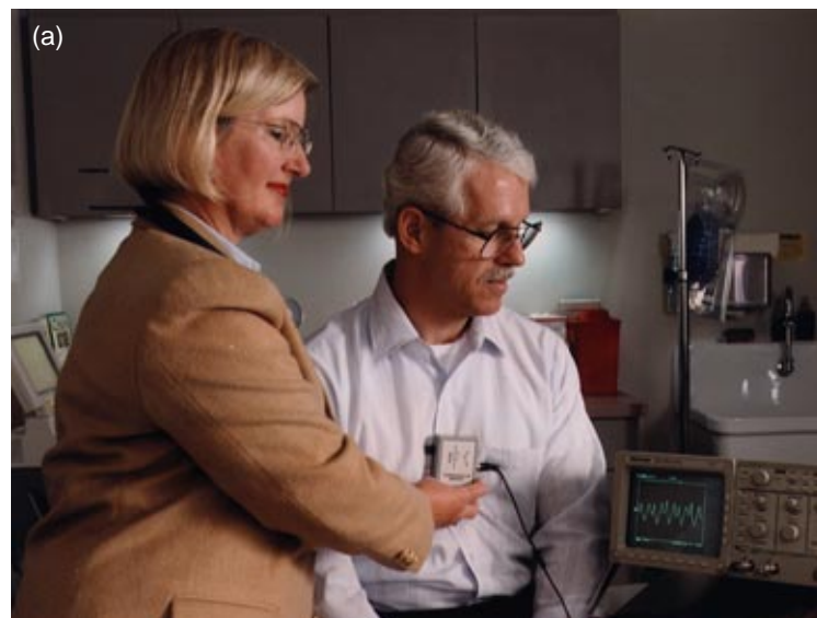
Figure 10. (a) An MIR cardiac monitor. (b) Its output (upper trace) is distinctly different from that obtained by a conventional EKG (lower trace). We are working with physicians to correlate the radar signals with physiological functions.
