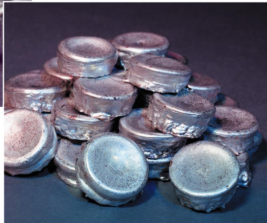
Enriched uranium produced at the Livermore pilot plant was collected as nuggets the size and thickness of several quarters. The nuggets were packed in 55-gallon drums for shipment to commercial fuel fabricators.
