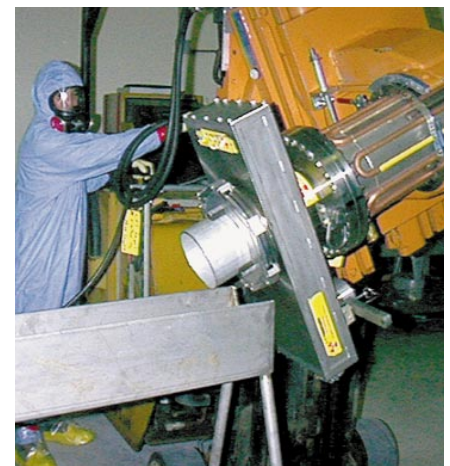
An operator removes enriched product from the separator withdrawal canister.
