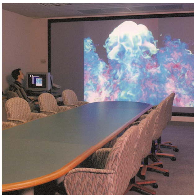
The power wall in the Assessment Theater (left) permits physicists to see ASCII codes in detail. On its screen is a simulation of two gases intermixing after being hit by a shock wave. At right, an operator uses projectors arranged in a 5 by 3 array to create and control the large, clear display.
