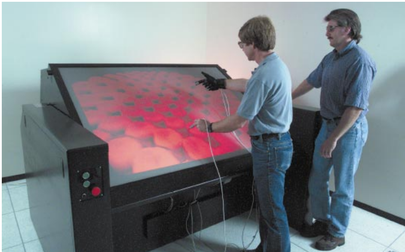
Livermore computer scientists test the usefulness of "data gloves" that allow the user to reach out and seemingly move and examine images. The gloves are being tested with a novel desktop display that is also under evaluation.
