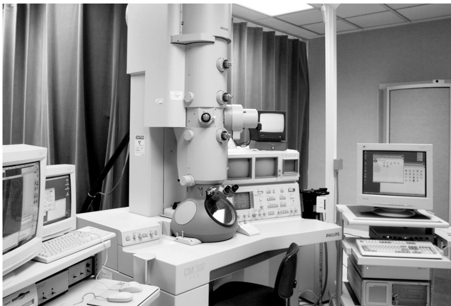
Metallurgists are probing the microstructure of actinides with a transmission electron microscope capable of near-atomic resolution.
