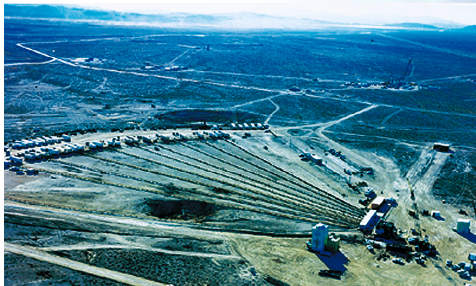
Aboveground diagnostic setup for an underground experiment at the Nevada Test Site. Data signals from a test explosion moved from the device, 300 meters downhole, up to the surface through cables, and the cables fanned out along the surface to trailers that housed instruments for reading the signals.
