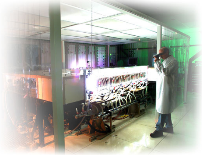
Laser technician Balbir Bhachu monitors the performance of the 13,000-watt solid-state heat-capacity laser during a low-power test. The prototype uses an electrical source to power flashlamps, which in turn pump nine neodymium-doped glass laser disks that release energy in pulses of laser light.
