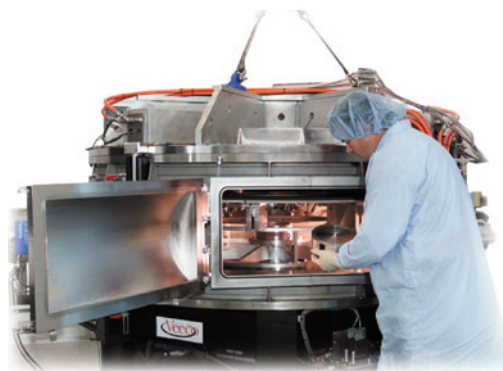
Process engineer Mark Schmidt places an optical substrate in the coating deposition chamber.
