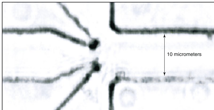
Olgica Bakajin is designing and fabricating this fast microfluidic mixer used for researching the kinetics of protein folding.
