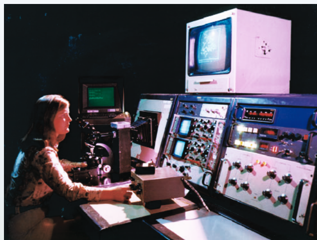
Bioengineers at Livermore combined mechanical skills with an understanding of biology to design the cytophotometric data converter (CYDAC), a highly sensitive diagnostic instrument that measures the amount of DNA in chromosomes. In this 1976 photograph, bioresearcher Linda Ashworth uses CYDAC to scan chromosomes from a mammalian cell.
