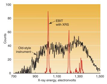
Data on charge-exchange-induced x-ray emissions supplied by electron beam ion trap (EBIT) experiments with the x-ray spectrometer (XRS) are enormously more detailed than data supplied by old-style detectors. This graph compares the data supplied by each instrument in registering x-ray emissions caused by charge-exchange reactions involving an ion of neon (Ne<sup>9+</sup>).
