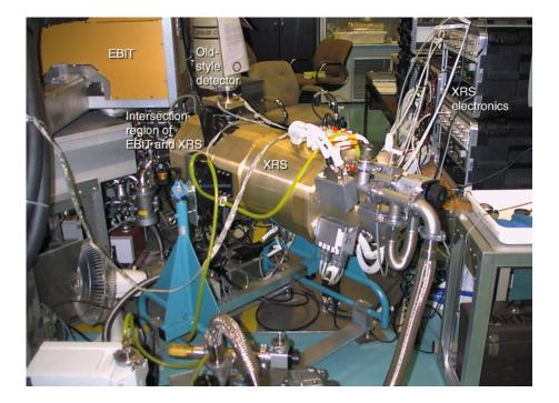
At Livermore's electron beam ion trap (EBIT) facility, scientists study the charge-exchange process and the effects of different ions and interaction gas molecules on the x-ray emission patterns recorded by the x-ray spectrometer (XRS) (front). The EBIT (in back) provides a source of ions to re-create solar wind particles. At the left is an old-style spectrometer. Also shown is the intersection of the XRS and EBIT.
