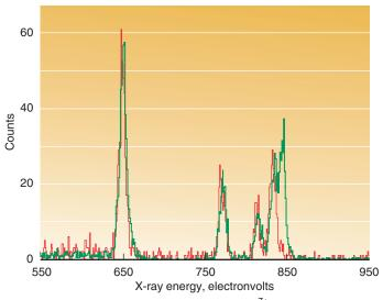
Plots of x-ray emissions from an ion of oxygen ( $O^{7+}$ ) caused by interactions of  $O^{8+}$  with methane (CH<sub>4</sub>, the green trace) or with nitrogen (N<sub>2</sub>, the red trace) reveal subtle changes in the x-ray emission lines when these different neutral gases collide with the heavy ions. The changes are found near 850 electronvolts.
