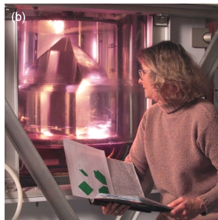
(a) An 8- by 8-micrometer scanned image of the face of a potassium dihydrogen phosphate (KDP) crystal. The morphology and dynamics of crystal growth are relevant to the National Ignition Facility (NIF) as well as to projects that study biomaterials. (b) An example of a large KDP crystal grown for the NIF laser.
