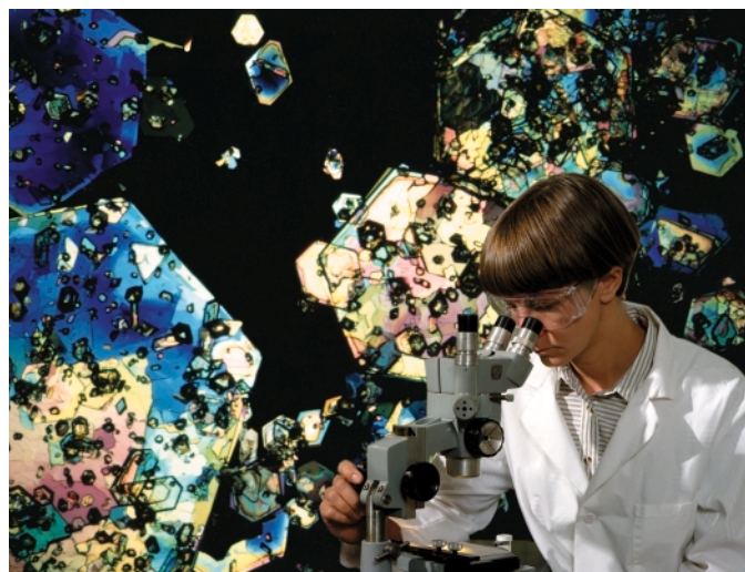
Fran Foltz examines crystals of the insensitive high explosive triamino-trinitrobenzene (TATB) under the microscope. The background shows TATB crystals at high magnification.
