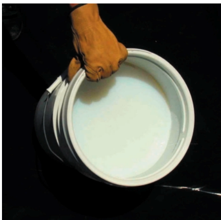
L-Gel is shipped premixed as a semisolid. It is reliefsed to a house-paint consistency by vigorously shaking it by hand or using a power stirrer.
