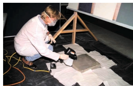
Researcher Paula Krauter applies L-Gel to "contaminated" panels of different materials to test the gel's effectiveness.
