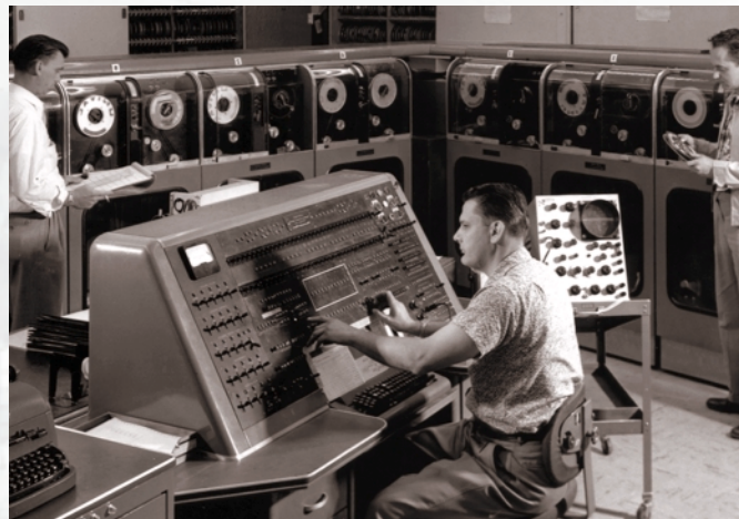
The Univac was the first computer to store information on magnetic tape. Running a program was a hands-on operation, with a physicist or programmer toggling console switches to execute the problem. Although highly accurate, the Univac was cantankerous, breaking down two or three times a day. Early workers regarded it as an "oversized toaster."
