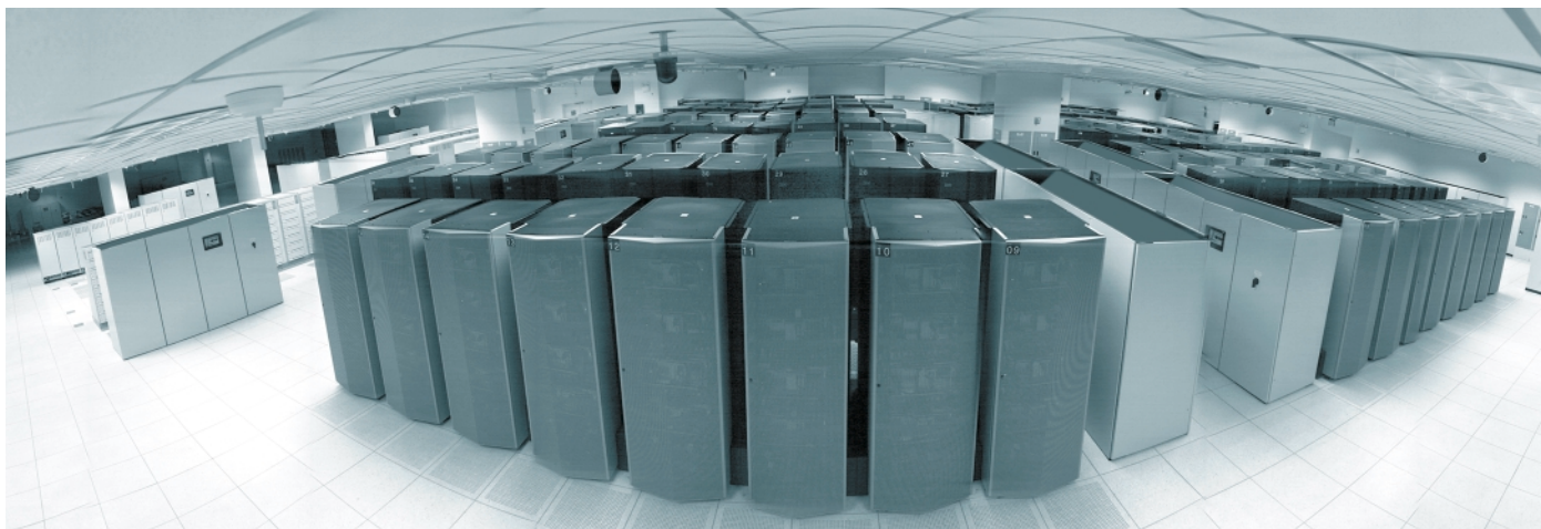
The ASCI White, with power to perform 12 trillion operations per second, was delivered to the Laboratory during the summer of 2000.
