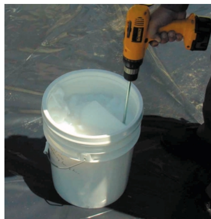
L-Gel is shipped premixed as a semisolid. It is reliefsied to a house-paint consistency by vigorously shaking it by hand or using a power stirrer.
