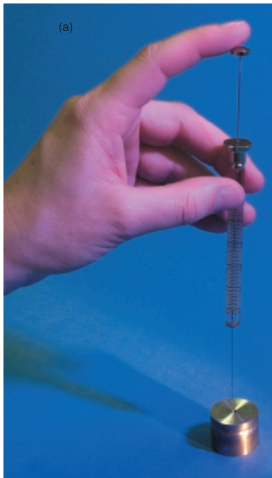
(a) A liquid sample is loaded into a capsule, which in turn will be placed into the chamber of Livermore's 6.2-meter-long light-gas gun. (b) A schematic of the gas gun in operation. A gunpowder explosion on the left pushes the piston, which pushes helium gas to open the rupture valve. The projectile then flies down the barrel of the gun to hit the target inside the gun's chamber.
