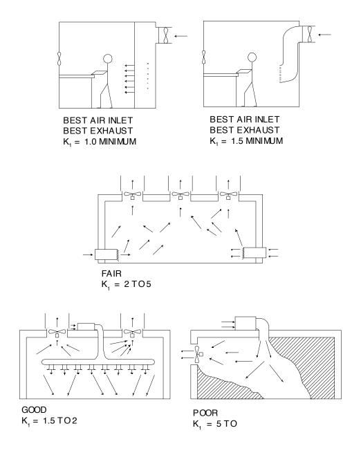
Figure 3.1: Typical K, Factors Based on Inlet and Exhaust Locations
