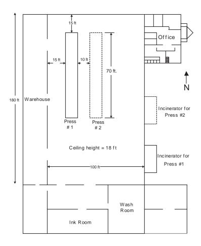
Figure 3.7: Example Plant Layout
