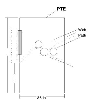
Figure 3.5: Unmanned PTE (Around One Station of a Coater)
