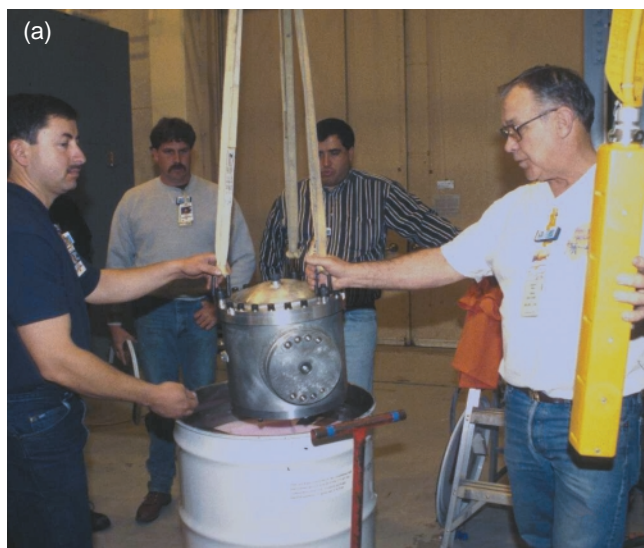
(a) Gerard Martinez of Los Alamos (left) and Richard Ring of Livermore remove the B61 test object from its shipping container. (b) The B61 test object is mounted on the carriage of the shock machine for a drop test. The shock test is part of the annual stockpile certification process.
