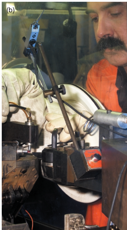
(a) Bill Poulos machines a plutonium part to be used in an experiment. (b) Ed Thomas sets up a tool on a Moore T lathe in preparation for computerized machining of plutonium parts. (c) Dale Tumlin inspects the gold that has been deposited on a glass slide. The thickness of the gold is 1.5 micrometers. All of these technicians are trained fissile material handlers.
