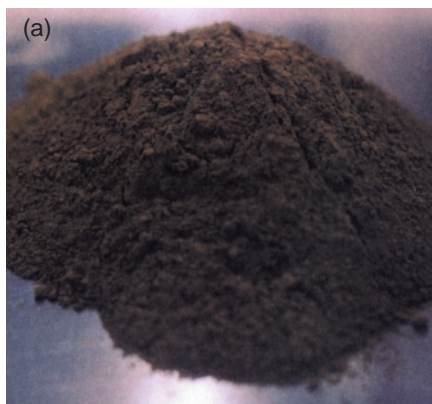
Livermore is developing the technology and the hardware to immobilize DOE's excess plutonium. (a) Plutonium oxide powder is blended into a ceramic material and then granulated, pressed, and baked to produce (b) ceramic "pucks" for long-term storage.
