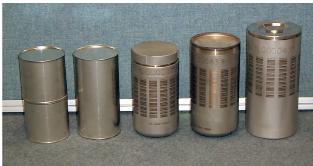
There are three configurations of the "convenience can" used for storing plutonium oxide and other excess plutonium metal. These three configurations are shown, from left, by the first stack of two cans, second can, and third can. Each convenience can will be crimp sealed or screw sealed and placed inside an inner can (fourth one from left), and it is then welded shut. The inner can is itself placed inside an outer can (fifth from left), which is also welded shut.
