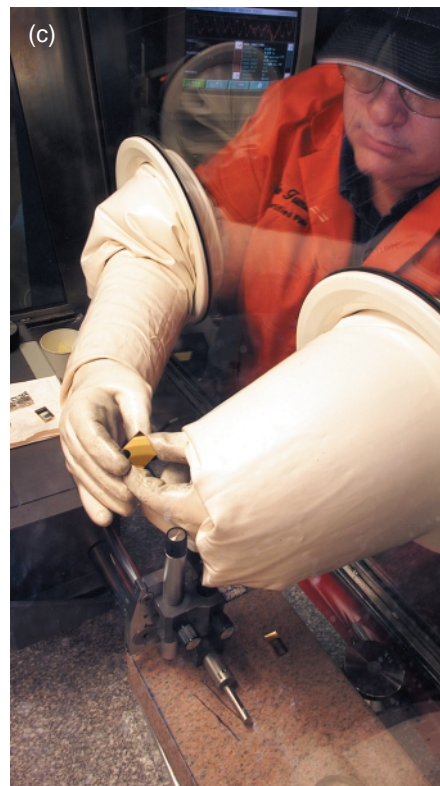
(a) Bill Poulos machines a plutonium part to be used in an experiment. (b) Ed Thomas sets up a tool on a Moore T lathe in preparation for computerized machining of plutonium parts. (c) Dale Tumlin inspects the gold that has been deposited on a glass slide. The thickness of the gold is 1.5 micrometers. All of these technicians are trained fissile material handlers.
